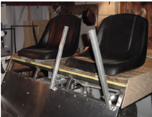
Installation of Seats and Splash Panels
