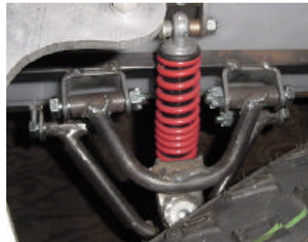
Installation of Front Suspension assembly
