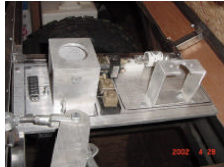
Installation of Electronics Module mount block
